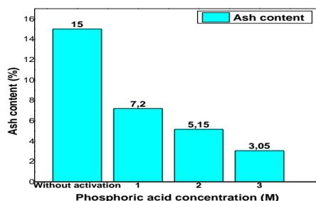
Figure 5. Ash content of activated carbon before and after activation.
