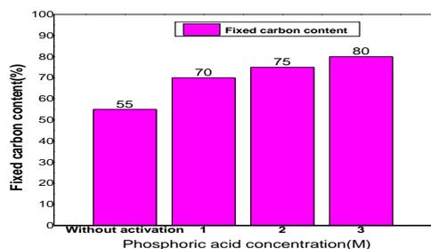
**Figure 6.** Fixed carbon content of activated carbon before and after activation.
