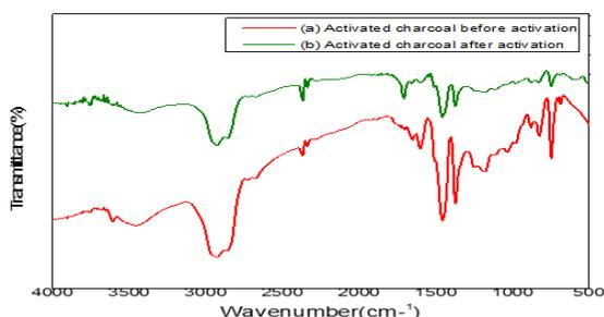
**Figure 1.** FTIR spectra of activated charcoal before and after chemical activation
