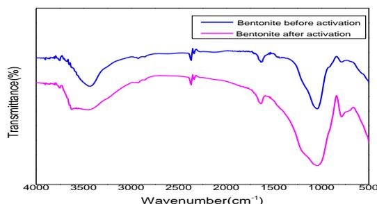
Figure 2. FTIR spectrum of bentonite before and after activation
