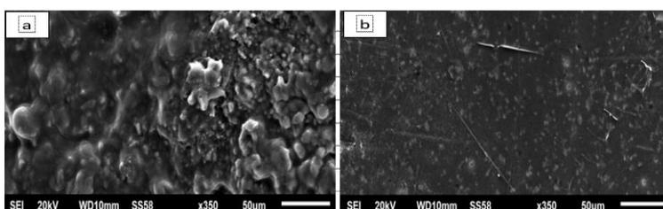
Figure 3a. SEM image of the bentonite and activated carbon composite before chemical activation.
